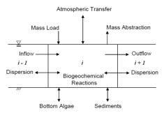
**Fig 4:** Processes included in the general mass balance in the modelling of QUAL2K water quality parameters for a segment without a tributary (Adapted from Chapra et al. 2006).
