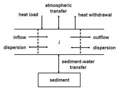
Fig 1: Heat balance for an element
