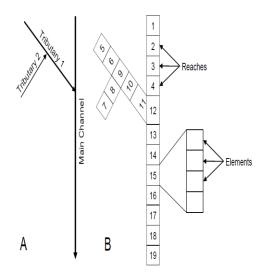
**Fig 2:** Transformation of a hypothetical river (A) into the QUAL2K representation of that river (B) (Adapted from Chapra et al. 2006).
